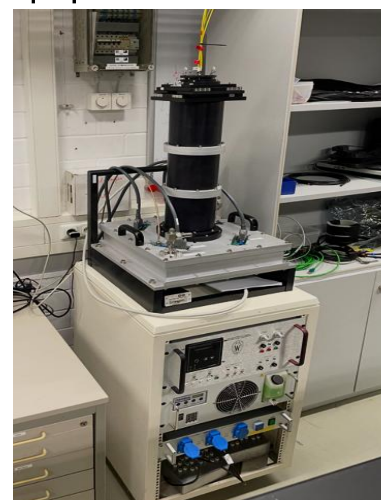
W7-X BES system with 64 channels (input fibers at the top of the image) [2]
