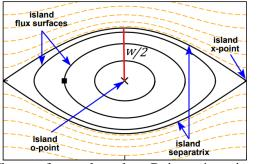
Flux surfaces plotted on Poincaré section with important island features labeled
