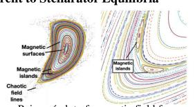
Poincaré plot of magnetic field from example NCSX coil set [1]
