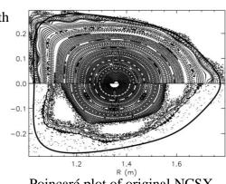
Poincaré plot of original NCSX magnetic field on bottom and "healed" magnetic field on top [2]
