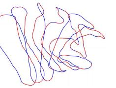
Free-boundary after helica flux optimization Original coils shown in red and helical flux optimized coils shown in blue. Small differences in coil geometry indicate high island sensitivity
