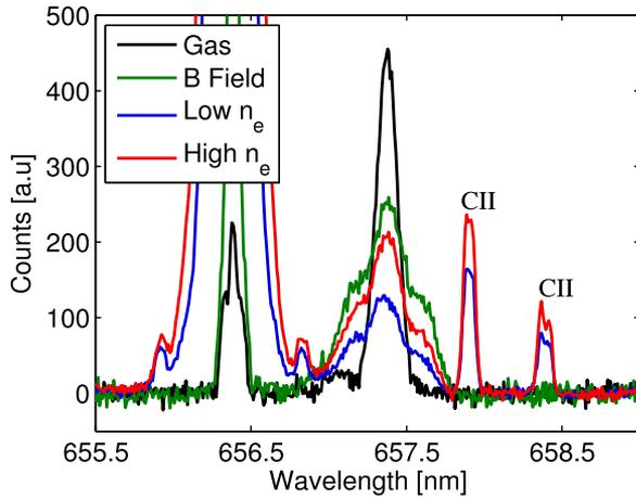
FIG. 3. Measured spectra of Doppler shifted  $H_\alpha$  emission from: beam into gas, beam into gas with magnetic field, and beam into plasma at low and high densities ( $2\text{-}4 \cdot 10^{18} \text{ m}^{-3}$ ).
