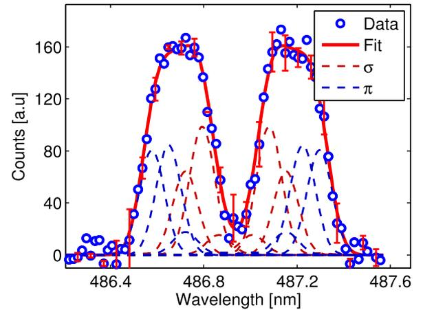
FIG. 2. Simulated  $H_\beta$  data with Gaussian noise and fit, included are the  $\sigma$  and  $\pi$  components.
