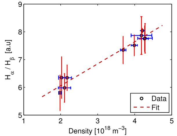
FIG. 5. Ratio of  $H_\alpha/H_\beta$  emission as a function of density.
