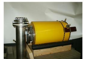
Diagnostic neutral beam ready to be installed on HSX
