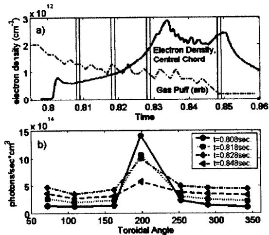
FIG. 6. (a) The density evolution (solid) and gas puff (--) of a discharge with a poorly conditioned vacuum vessel, and (b) the toroidal asymmetry in  $H_{\alpha}$  emission at different times in the discharge. The times for the profiles correspond to the shaded areas of the time trace.
