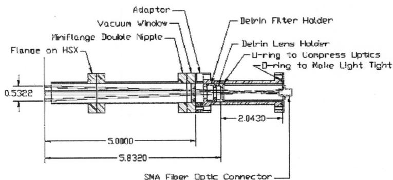
FIG. 3. Design of the collection optics of the  $H_{\alpha}$  detector.
