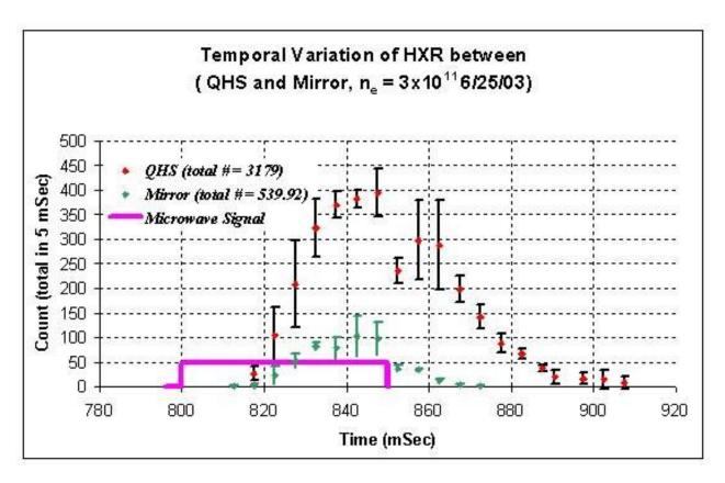
• Intensity increases till gyrotron turn-off, then decreases with 13 ms time constant for QHS, 5 ms for Mirror; virtually no hard x-ray counts for anti-Mirror
