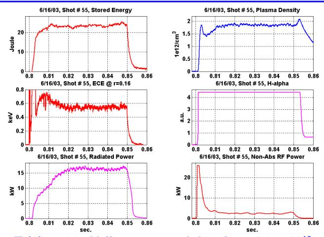
$T_e(0) \sim 600$  eV, line averaged density  $\sim 1.8 \times 10^{18}$  m<sup>-3</sup> W  $\sim 25$  J,  $P_{rad} \sim 17$  kW (40 kW injected)
