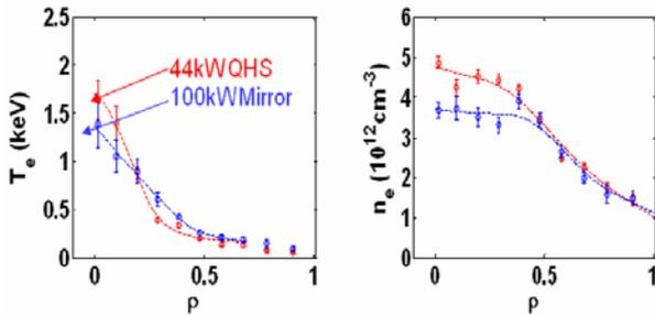
Fig.2 Profiles demonstrating that 2.3 times the injected power is required in Mirror to minimize the difference in the temperature profiles.
