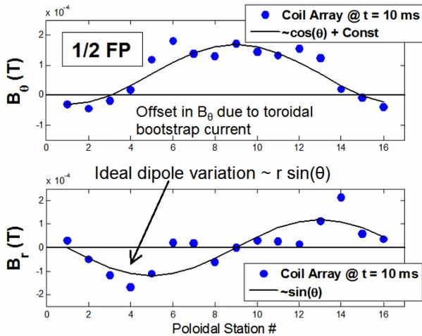
Fig. 7. Measured poloidal and radial magnetic fields at 16 poloidal stations.
