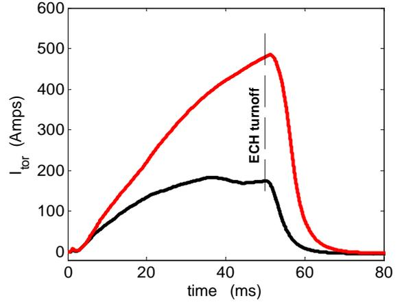
Fig. 3. Time evolution of the toroidal current. Heating resonance: off-axis (black), near-axis (red).
