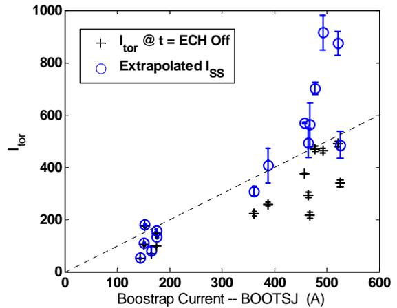
Fig. 8. Measured and projected values of total bootstrap current vs. estimated bootstrap current. Estimate is calculated by BOOTSJ.
