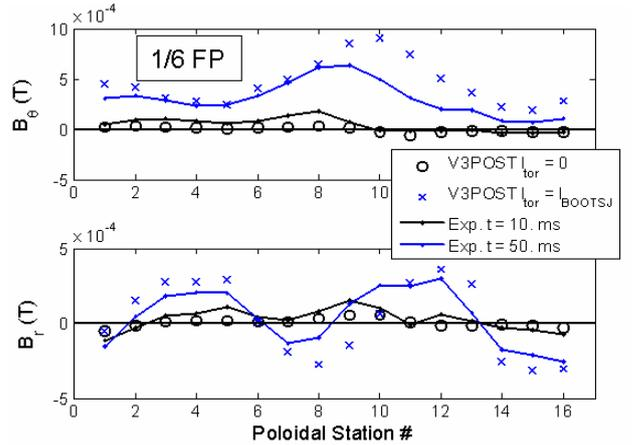
Fig. 12. Magnetic diagnostic responses at a toroidal location of 1/6 field period.
