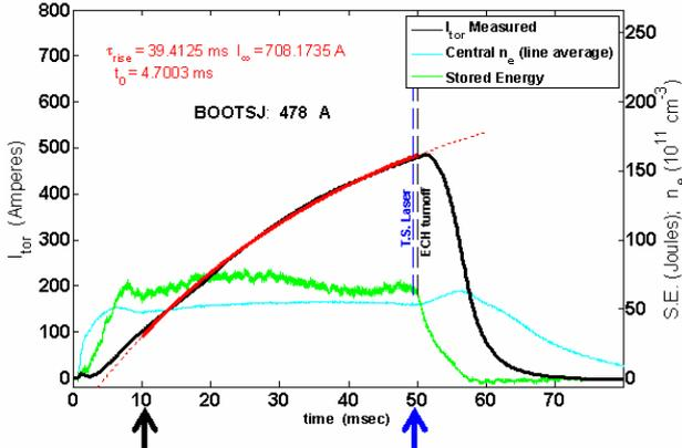
Fig. 9. Time evolution of toroidal current, stored energy, and line-averaged central  $n_e$
