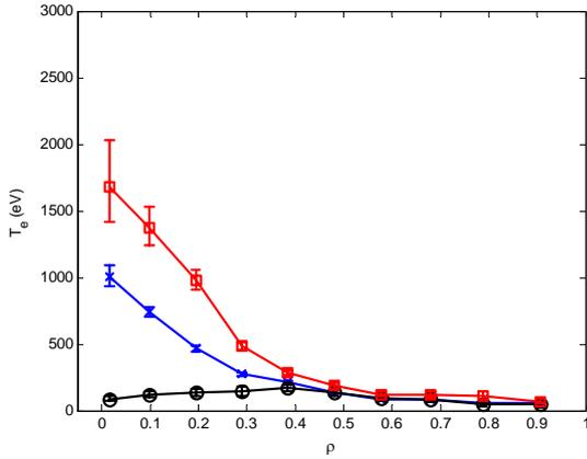
Fig. 1. Electron temperature radial profiles. The various profiles are achieved by varying the electron-cyclotron resonance heating location. ECRH power  $\sim 44$  kW (launched).
