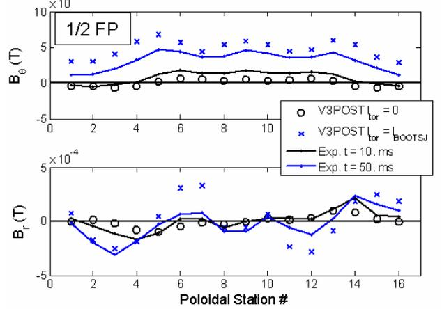
Fig. 11. Magnetic diagnostic responses, measured and calculated (V3FIT results marked as V3POST).
