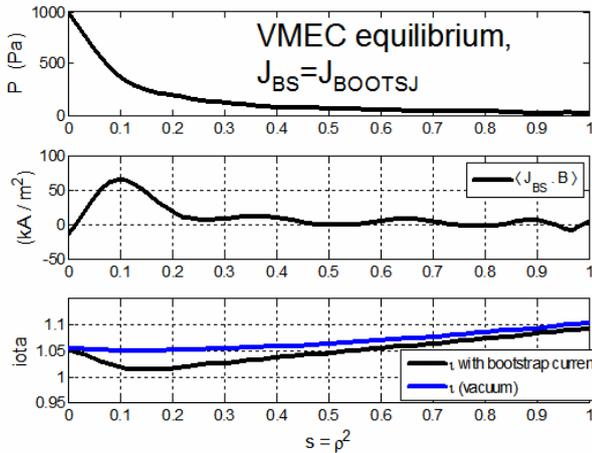
Fig. 10. Radial (VMEC 's') profiles of plasma pressure, bootstrap current and rotational transform. The vacuum transform is also shown.
