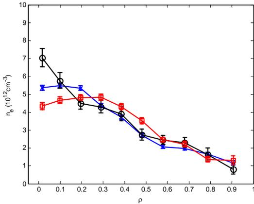
Fig. 2. Electron density profiles. The line-averaged central density is  $4.7 \pm 0.3 \times 10^{18} \text{ cm}^{-3}$  in each case.
