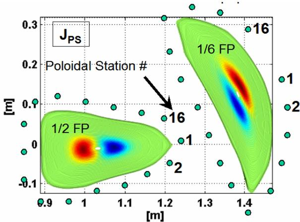
Fig. 6. Pfirsch-Schlüter current density at two toroidal locations and a sketch of the location of the dB/dt triplets.
