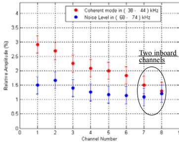
Fig.6 Amplitude of plasma density fluctuations measured by ECE radiometer
