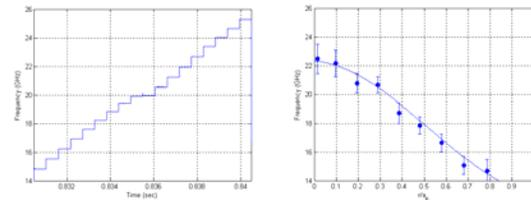
Fig.8 Probing beam frequency sweep and X-wave cut-off frequency in HSX plasma
