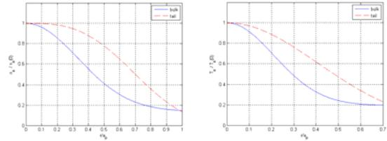
Fig.3 Normalized  $N_e$  and  $T_e$  profiles for bulk and tail plasmas
