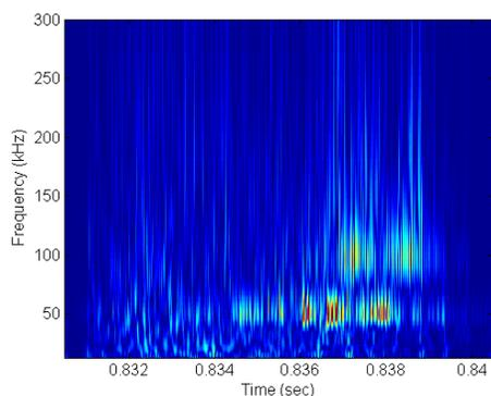
Fig.9 Wavelet coefficients in QHS (one full sweep of the reflectometer)
