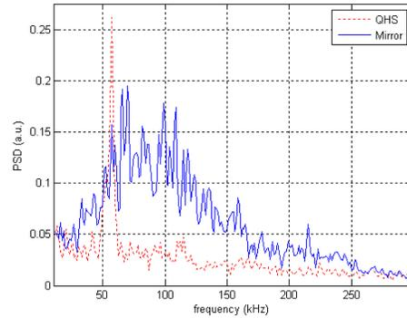
Fig.7 FFT of the reflectometer signals in QHS and 10% Mirror
