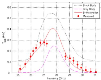
Fig.2 Measured ECE spectrum and the fit based on Bi-Maxwellian plasma model
