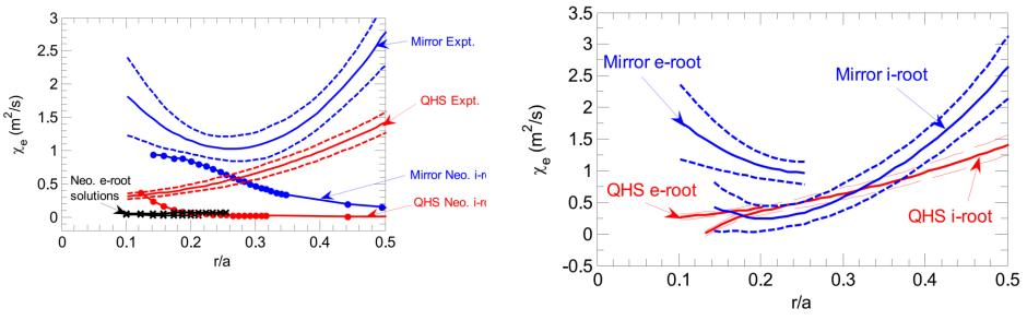
Lore 2010 ECRH at B = 1.0 T: Ambiguous whether QHS or Mirror configuration has lower turbulent transport. Mirror configuration = 10% Flip14
