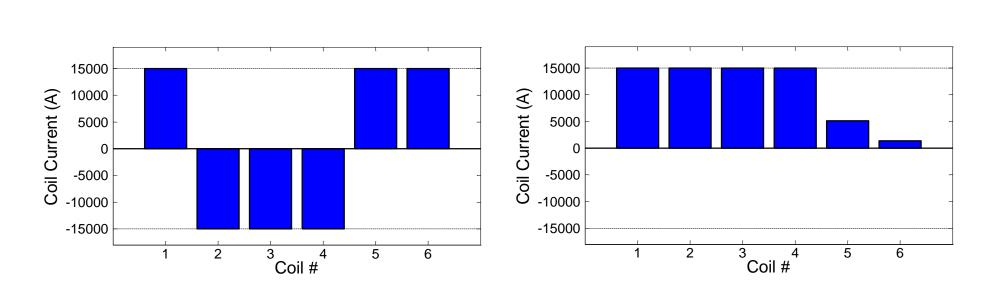
Flip14 (10%) is the normal configuration we use to degrade the quasisymmetry (left). Coil configuration on right is result of trying to maximize the proxy function.
