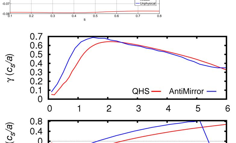
Linear GENE calculation shows that growth rate in AntiMirror configuration is worse than QHS, contrary to simple proxy result:  $a/L_{Te} = 1$ ,  $a/L_{n} = 2$ ,  $a/L_{Ti} = 0$ ,  $T_{e} = T_{i}$
