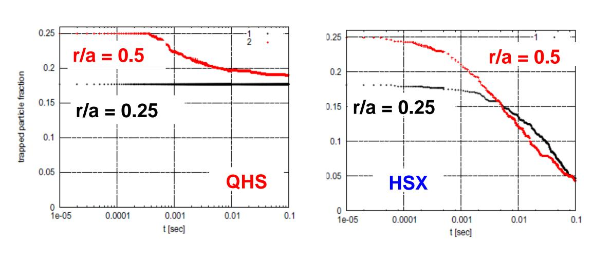
• QHS is the original Nührenberg & Zille (1988). HSX is described by finite coils, which introduce additional minima in |B|. QHS & HSX both scaled to B = 5T, a = 1.6 m.
