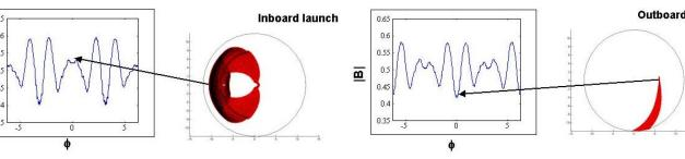
• When electrons are launched at the inboard side (local maximum of the magnetic field) they are trapped with their orbits deviation from flux surface being large compared to QHS and Mirror cases. • When electrons are launched at the outboard side (bottom of the magnetic well) they are in direct loss orbit.
