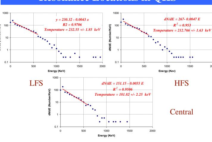
As predicted before from the energetic electrons drift orbit analysis in QHS (at  $n_e = 4 \times 10^{11} \text{ cm}^{-3}$ ), there is nearly no difference in hard x-ray emission at different resonance location.
