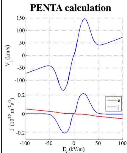
Helical resonance would appear as a sudden change in electrode current and parallel velocity.
