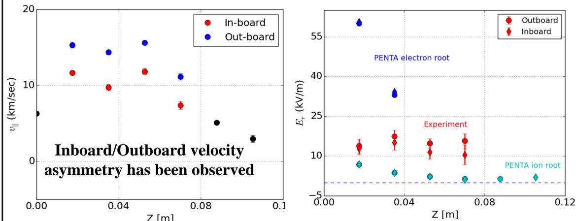
The  $E_r$  calculated from PS flows is between Electron and Ion roots calculated by PENTA, higher than that previously obtained from radial force balance.
