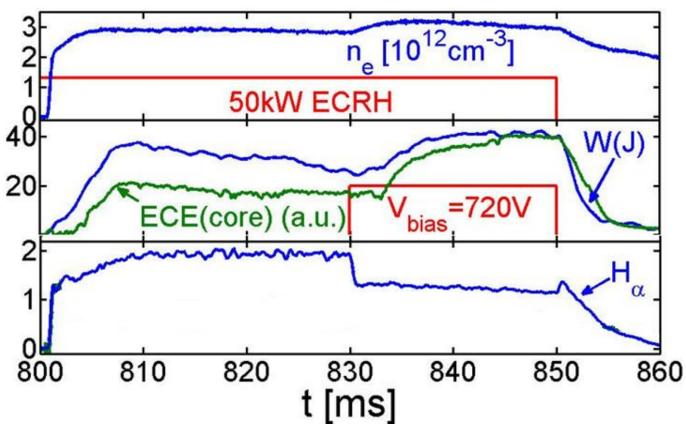
Biased electrode discharges in HSX show H-mode like characteristics. However, expected change in electrode current and large change in parallel flow haven't been observed during bias.
