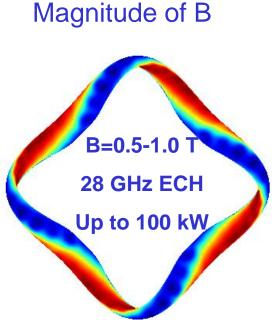
HSX has a helical axis of symmetry in |B| and a resulting very low level of neoclassical transport
