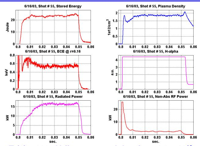
$T_e(0) \sim 600$  eV, line averaged density  $\sim 1.8 \times 10^{12}$  m<sup>-3</sup> W  $\sim 25$  J,  $P_{rad} \sim 17$  kW (50 kW injected)
