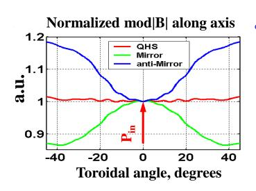
Mirror configurations in HSX are produced with auxiliary coils in which an additional toroidal mirror term is added to the magnetic field spectrum
