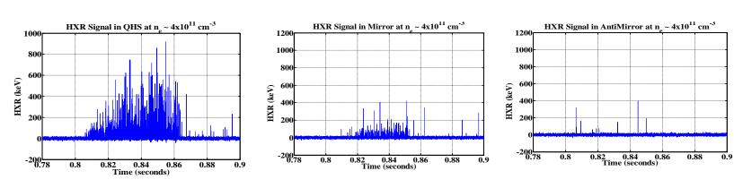
Energetic electrons produced by 2<sup>nd</sup> harmonic ECH are well confined with quasisymmetry and lead to intense hard x-ray signals (See Poster by Abdou –this session)
