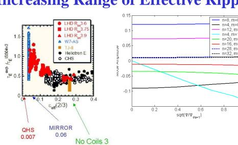
By varying the current in modular coil type 3 (of 6 per period) a broad range of effective ripple can be achieved with well-formed magnetic
