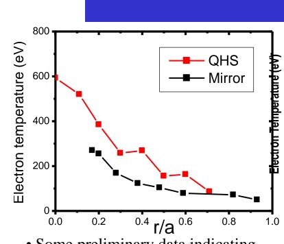
• Some preliminary data indicating difference in QHS/Mirror T<sub>e</sub> profiles Neoclassical thermal conductivity i QHS is about 3 orders of magnitude
