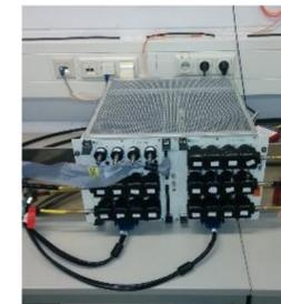
The filterscope system has been installed and calibrated and is ready for plasma data acquisition at W7-X.
