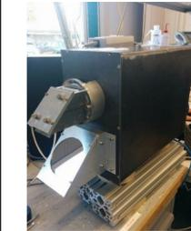
A beamsplitter (Ge) allows IR to penetrate and reflects the visible. This allows the two cameras to share the same limiter view, providing simultaneous measurements of heat and particle flux.
