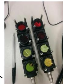
Beamsplitters allow each spectral channel to be split into 4 spectral channels, providing more information without adjustment.
