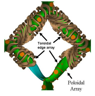
Toroidal edge array at same field period locations will be used to detect the toroidal mode number, n, at high and low field side of the plasma.
