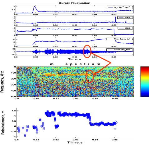
•At about 0.2 x 10<sup>12</sup> cm<sup>-3</sup> in QHS-Central Resonance, there exists a mode transition from m = 1 to m = 0.
