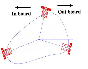
Using the results of coherent and bursty fluctuation measurements, 3 rotatable magnetic probes will be used to measure the poloidal mode spectrum up to m = 1.
