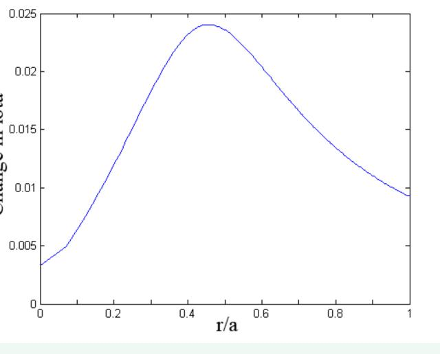
Change in rotational transform due to 400A bootstrap current – a VMEC calculation.  $\Delta \gamma_{max} \sim 1.4^o$
