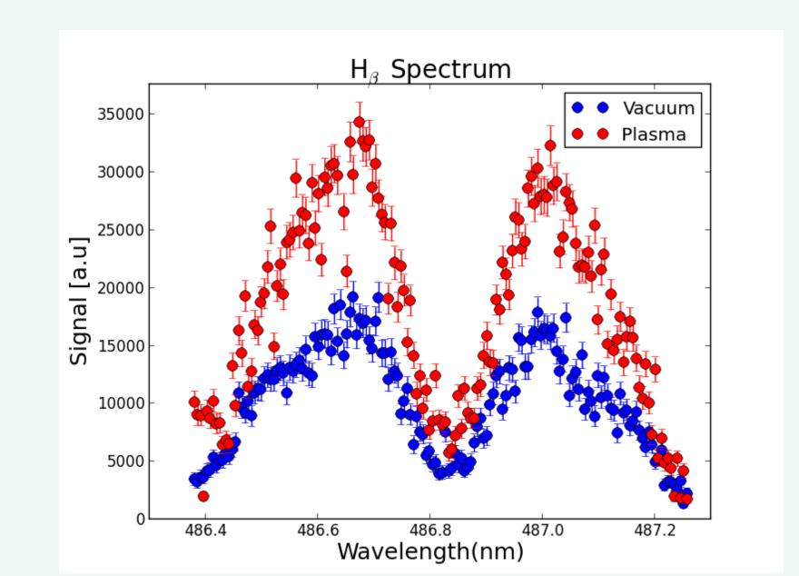
f=1m Czerny-Turner spectrometer, 19x200 micron fibers, 2160 g/mm grating
