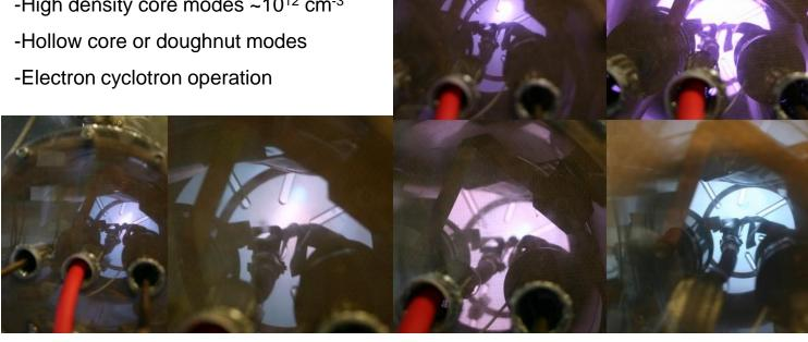
Instabilities were picked up on the Langmuir probe, as well as with a photodiode and an antenna:
