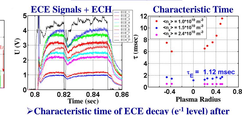
the gyrotron turn-off decreases with plasma density --- at  $1 \cdot 10^{18}$  m<sup>-3</sup> the decay is slower than energy confinement time from the diamagnetic loop ( $\tau_E \approx 1 \text{ msec}$ ) and faster at 2.4·10<sup>18</sup> m<sup>-3</sup>
