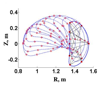
> 240 rays are launched into the plasma from 80 points distributed uniformly across and along the machine at random angles
