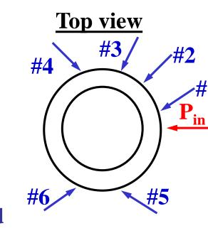
Six absolutely calibrated µ-wave detectors are installed around the HSX at  $6^{\circ}$ ,  $36^{\circ}$ ,  $\pm 70^{\circ}$  and  $\pm$ 100° (0.2 m, 0.9 m, 1.6 m and 2.6 m away from μ-wave power launch port, respectively). #3 and **#5, #4 and #6 are located** symmetrically to the ECRH
