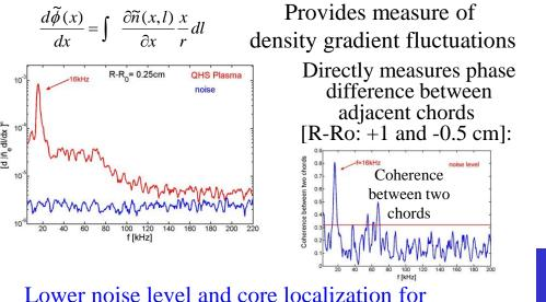
differential interferometer measurement
