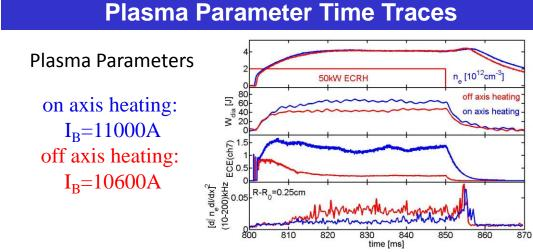
Input ECH power are similar, but significantly lower stored energy for off-axis heated plasma. Measured density fluctuations are of larger amplitude and at higher frequency for off-axis heating
