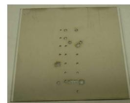
A laser blow-off target that has been used on HSX
