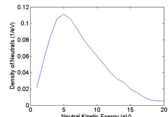
The neutral spectrum for a 2 μm aluminum film illuminated with a 7 J/cm<sup>2</sup> laser pulse [Breton '80]
