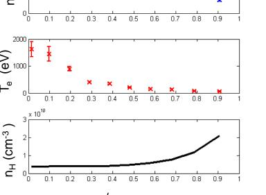
• N<sub>H</sub> is calculated using the DEGAS neutral gas modeling code and measurements
